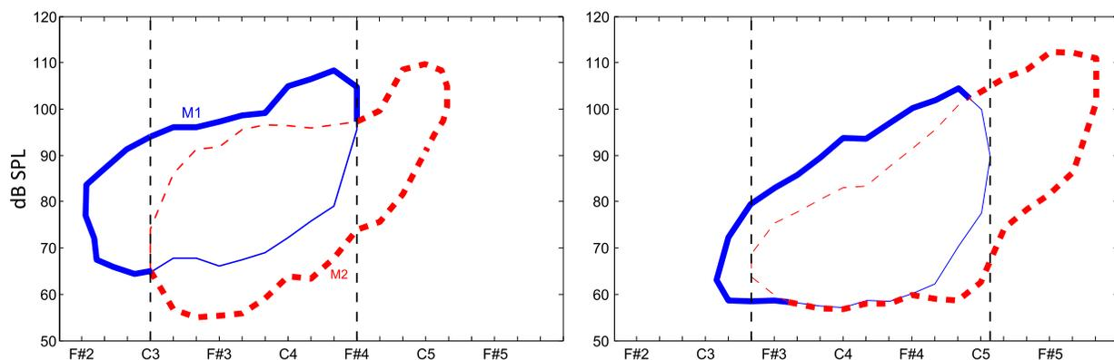
**FIGURE 1.** VRPs by laryngeal mechanism of a counter-tenor (*left*) and a mezzo-soprano (*right*). M1: connected line, M2: dotted line, vowel: /a/. The shared portion of both zones is drawn using thin lines, whereas the unshared portions of M1 and M2 are drawn with thick lines. VRP, voice range profile; SPL, sound pressure level.
