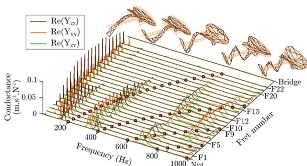
FIG. 7. (Color online) Out-of-plane ( $ZZ$ ), in-plane ( $YY$ ), and cross ( $ZY$ ) conductance along the G3 string's axis: at every fret and at the bridge. For each fret, circle and squares denote the string's fundamental frequency and partials respectively, for the considered bandwidth. A modal analysis allows us to identify the modes for each out-of-plane conductance peak, above which the corresponding mode shapes are drawn.
