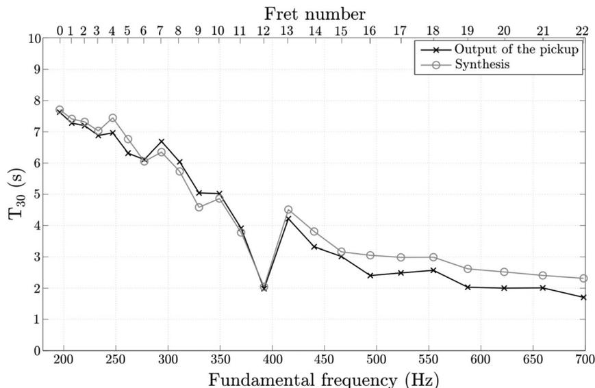
FIG. 12. T<sub>30</sub> for each fret of the G3 string. Gray circles indicate T<sub>30</sub> values computed from the synthesized signal. Black crosses indicate T<sub>30</sub> values computed directly from the output signal of the pickup.
