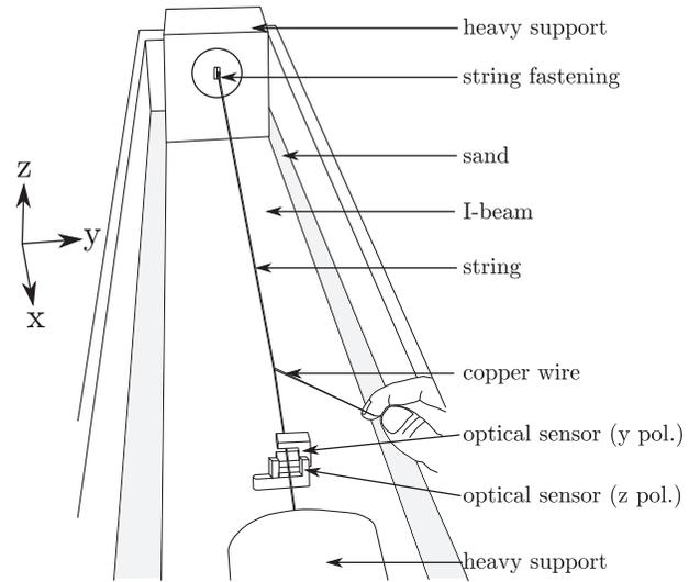
FIG. 4. Sketch of the measurement setup for the isolated string. The string is stretched between two heavy supports at playing tension and length. Two optical sensors measure each transverse ( $y$  and  $z$ ) polarization. The string is excited with the wire-breaking method. Clamps firmly attach the string's heavy supports as well as the optical sensors' supports to a heavy I-beam filled with sand, and are not drawn here for clarity reason.
