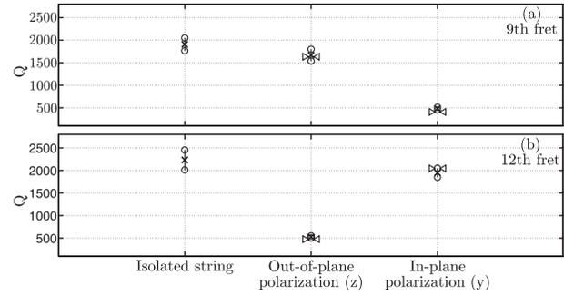
FIG. 9. Identified  $Q$  factor for the fundamental frequency of the note played at 9th fret (a) and 12th fret (b) of the G3 string. Both polarizations' results for the mounted string are compared to the isolated string. Circles and crosses indicate mean values and expanded uncertainty (95% confidence interval) respectively of 15 measurements. The arrows point out the  $Q$  value computed by the model of Eq. (20) with the isolated-string  $Q$  factors and the conductance values.
