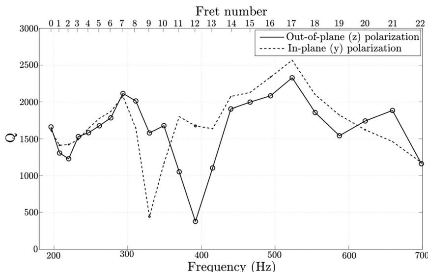
FIG. 11. Identified  $Q$  values associated with the fundamental frequency of both string polarizations. The analyzed signal is the output of the pickup, for each note played on the G3 string mounted on the guitar. Solid line is for the out-of-plane ( $z$ ) polarization and dashed line for the in-plane ( $y$ ) polarization. For each fret, circles' radii indicate the amplitude of the polarizations, normalized to the amplitude of the  $z$ -polarization.
