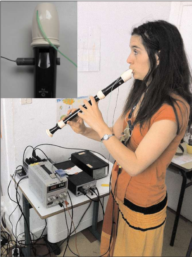
Figure 5. Experimental setup with the adapted alto Zen-On recorder, allowing the measurement of both the pressure in the mouth of the recorder player and the acoustic pressure under the labium.
