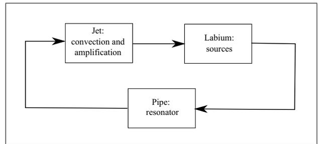
Figure 1. General description of flute operation as three independent blocks coupled together.
