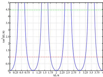
Figure 6: Position of the resonance frequencies in a graphical resolution of equation 9
