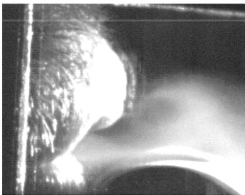
Figure 11: Lateral view from the lips of a flutist playing a flauta de chinos. It shows the characteristic openness of the lips and the turbulent structure of the air jet, which has been stained with smoke for visualization.
