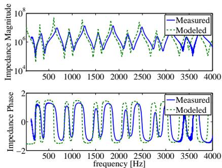
Figure 3: Comparison between the impedance measured and modeled for the *puntera*
