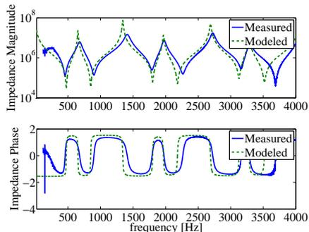
Figure 4: Comparison between the impedance measured and modeled for the *catarra*
