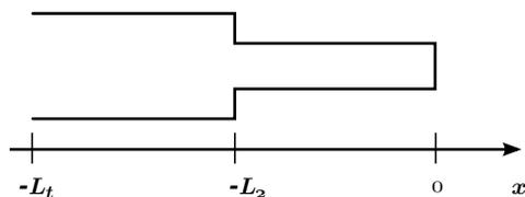
Figure 2: One-dimension model of the flute resonator. The embouchure is located at  $-L_t$
