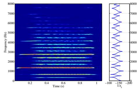
Figure 8: Spectrogram of the radiated sound from a *segundera*
