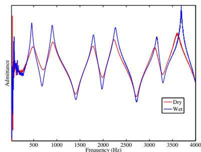
Figure 5: Measured input admittance comparison between a dry flauta (red) and a wet flute (blue). The larger amplitude observed in the wet pipe, due to the porosity reduction of the interior walls, allows for an easier sound production.
