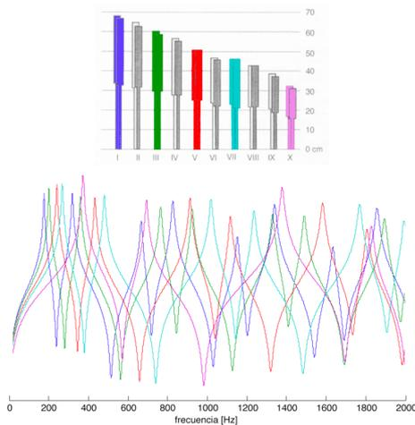
Figure 10: Ensemble of flutes with the detail of the complex tube geometry (top, from (de Arce 1998)) and the admittance of entry (below). For clarity of the representation, the plot includes the admittance of a subset of the flutes, which are individualized using a similar color in both graphs. Note how the sound of the ensemble fills much of the spectrum.
