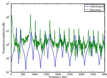
Figure 7: Comparison between the admittance model and the radiated spectrum for a *flauta puntera*). The spectrum and the admittance are both normalized in order to display them on the same figure
