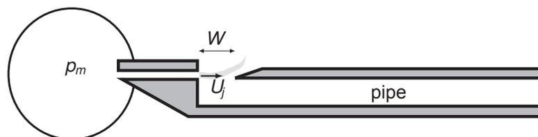
Figure 1: Simplified representation of a recorder, showing the pressure  $p_m$  in the mouth of the player and the jet velocity  $U_j$ .
