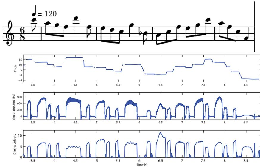
Figure 2: Score and raw data recorded while playing Teleman excerpt on an alto recorder. The pitch detected is plotted in semitones relative to A 440 Hz. The dimensionless jet velocity is calculated using the detected pitch and the distance  $W$  from the channel exit to the labium.
