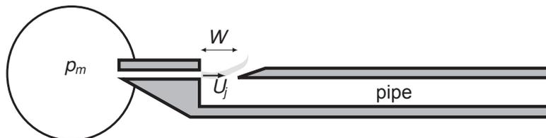
Figure 1: Simplified representation of a recorder, showing the pressure  $p_m$  in the mouth of the player and the jet velocity  $U_j$ .
