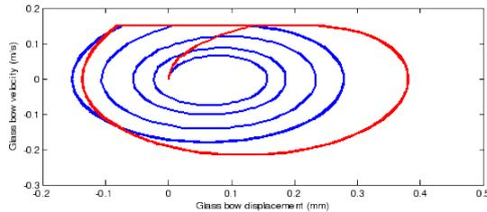
Figure 8: Limit cycles depending on finger force and velocity (blue:  $N = 10N, V = 0.15m/s$  / red:  $N = 20N, V = 0.15m/s$ )
