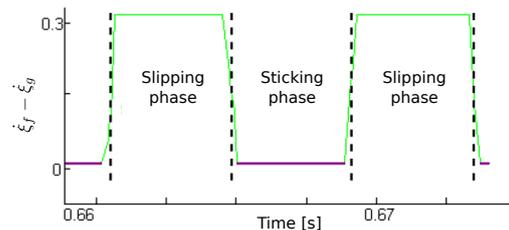
Figure 6: Relative velocity [m/s] between the finger and the glass bow versus time
