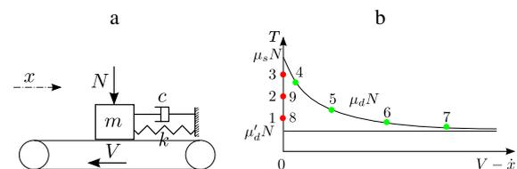
Figure 7: a) Single degree of freedom model and b) associated friction law
