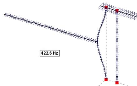
Figure 4: Modal shape of the main flexural mode of the resonator involved when playing the Cristal Baschet
