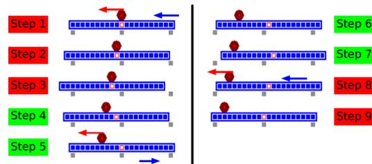
Figure 9: Stick-slip phenomenon occurring between the finger and the glass bow. Each of these steps are positioned on the friction law curve in Figure 7-b
