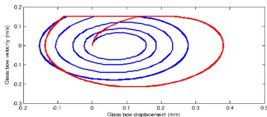
Figure 8: Limit cycles depending on finger force and velocity (blue:  $N = 10N, V = 0.15m/s$  / red:  $N = 20N, V = 0.15m/s$ )
