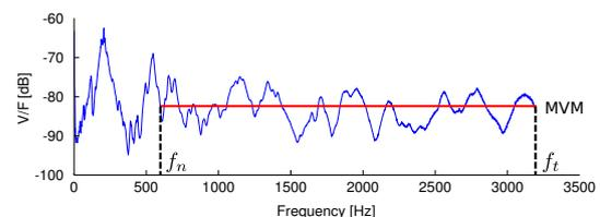
Figure 2: Mobility measured on the harp's soundboard and computed mean-value of the mobility (MVM)
