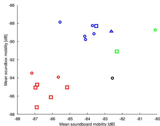
Figure 5: MVM of the sound-box versus MVM of the soundboard for 17 contemporary harps. Color corresponds to each harp maker and the marker to each harp's model: harp maker 1 - model A ( $\circ$ ), harp maker 2 - model A ( $\circ$ ) - model B ( $\square$ ), harp maker 3 - model A ( $\circ$ ) - model B ( $\square$ ), harp maker 4 - model A ( $\circ$ ) - model B ( $\square$ ) - model C ( $\triangle$ ).
