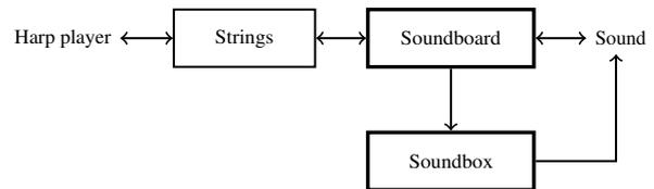
Figure 1: Schematic diagram of the harp's acoustical behavior
