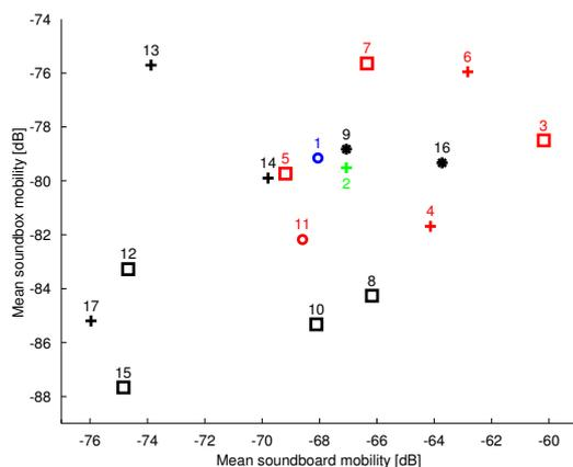
Figure 4: MVM of the sound-box versus MVM of the soundboard for the 17 historical harps described in Table 1. The number corresponds to the harps of Table 1, the color reports to each harp maker "family" and the marker to each harp maker: Saunier ( $\circ$ ), Louvet ( $+$ ), Cousineau G ( $\square$ ), Cousineau G et J-G ( $+$ ), Cousineau J-G ( $\circ$ ), Erard & Cie ( $\square$ ), Erard Frères ( $*$ ), Erard Sébastien ( $+$ ).
