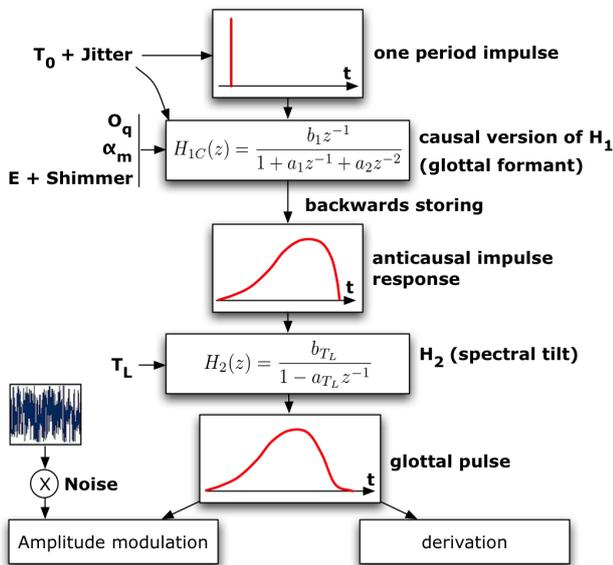
**Figure 4: Framework of RT-CALM algorithm, allowing real-time synthesis of glottal pulses based on causal-anticausal linear model.**
