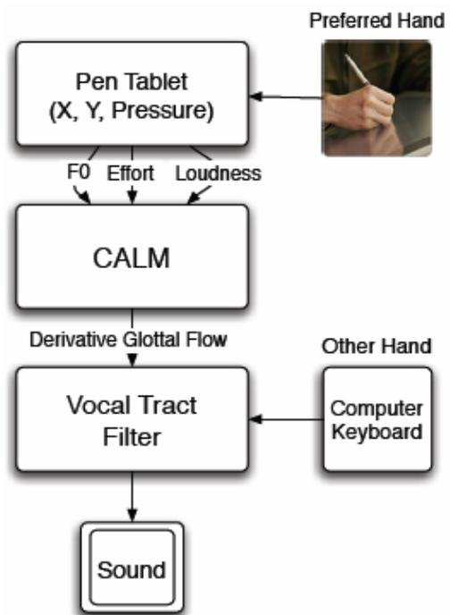
Figure 3: Instrument 3. graphic tablet controlled CALM synthesizer.
