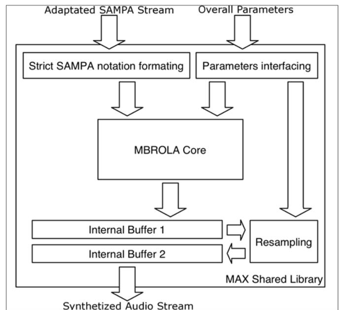
As shown in Figure 8, we can separate the possible requests in two main channels. On one side, there is parameter modification, which influences the internal state of the synthesizer. On the other side, there is the phonetic/prosodic stream, which generates speech instantaneously.
