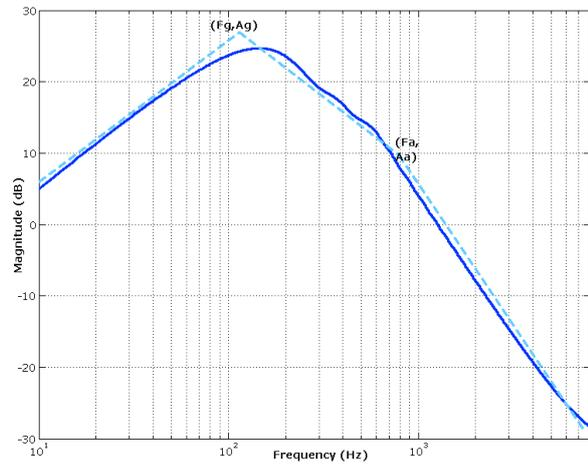
Figure 2: Amplitude spectrum of the glottal flow derivative: illustration of glottal formant ( $F_g, A_g$ ) and spectral tilt ( $F_a, A_a$ ).
