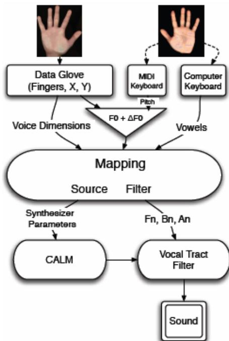
Figure 2: Instrument 2. Data glove controlled CALM synthesizer.
