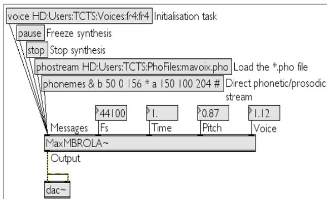
The MBROLA engine can also be stopped (*Messages* inlet). That function flushes the phonetic/prosodic content, stops the synthesis process and sets all the internal parameters to their default values. The diphone database remains loaded.
