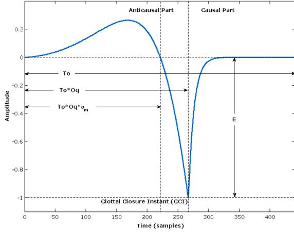
Figure 3: Time-domain representation of derivated glottal pulse: anticausal and causal parts, respectively on the left and right of the glottal closure instant.
