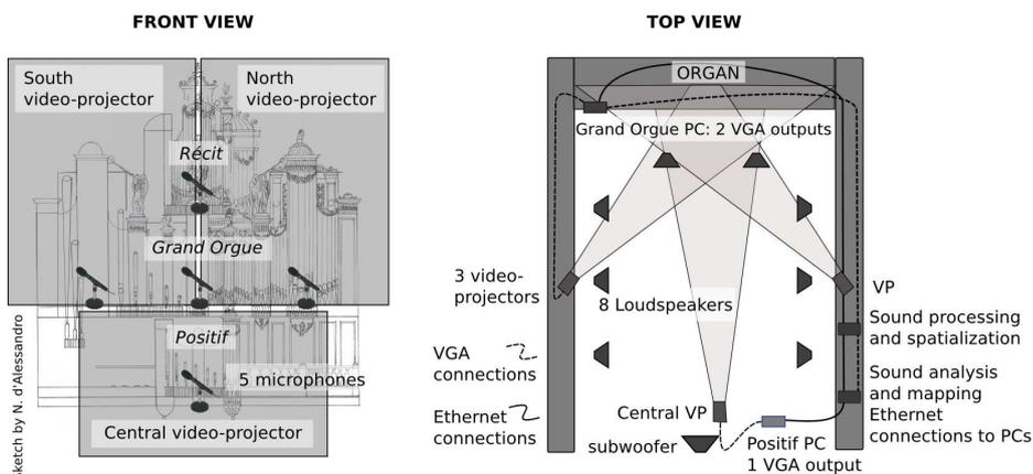
Fig. 2. Architecture of the installation: sound capture and video-projection
